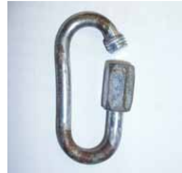
Link bent and rusted.
