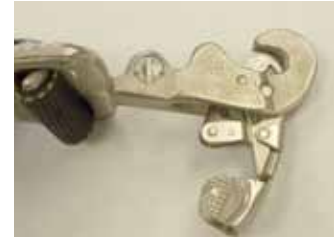
Spring broken, snap stays in open position.
