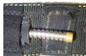
Housing out of place, tacking missing.
