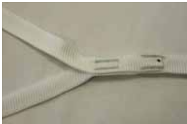
Bartacks secure, tubular in good condition.
