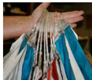
Lines out of trim.
