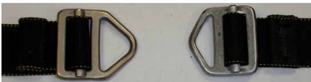
Shallow V should be replaced.
