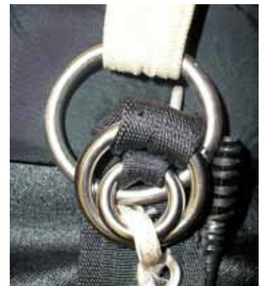
Large ring not round, around both smaller rings. Loop through both small rings.
