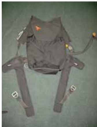
No holes, tears, or broken stitches.
