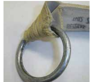
Fraying ring attachment point.
