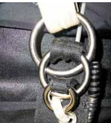
Properly routed and in good condition.
