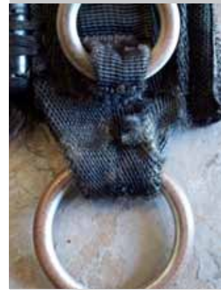
Webbing worn and fraying.
