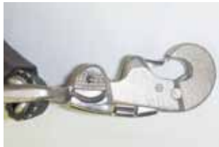
Snaps close completely. Not bent or broken.
