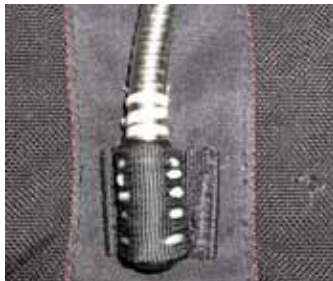
Tacking secure on drogue riser.
