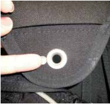
Fingernail doesn't slide under rim.
