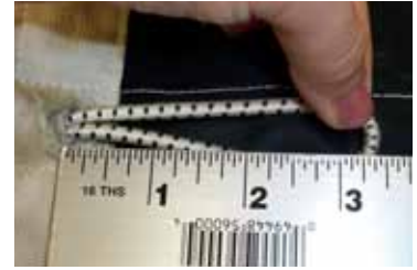
Shock cord loops stretched out. Missing Grommet.
